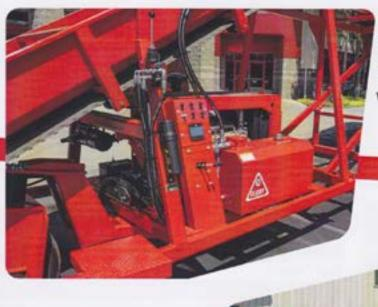
A powered drive wheel with a large flotation tire and smooth steering helps position the 3690 where you need it
